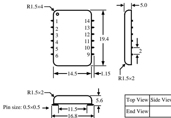
Figure 8 Dimensions of the SMT Package Controller
