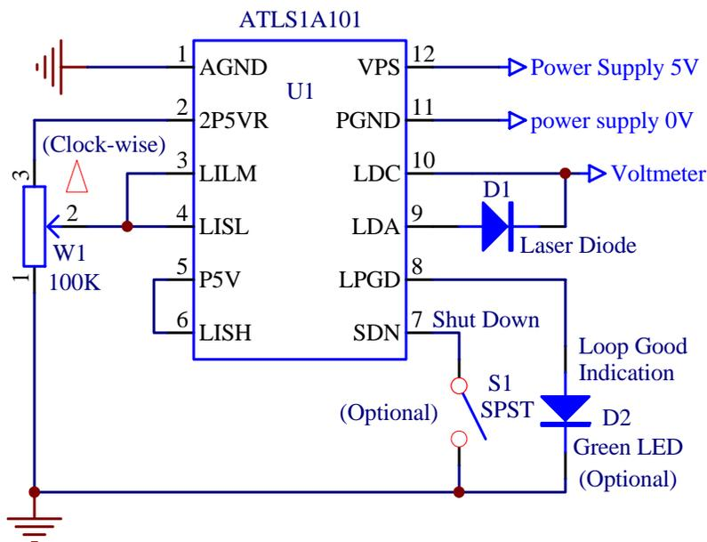
Figure 2 A Typical Stand-alone Application Schematic
