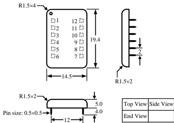
Figure 6 Dimensions of the DIP Package Controller
