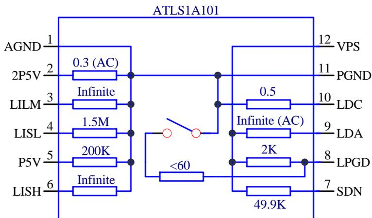
Figure 4 Equivalent Internal Circuits
